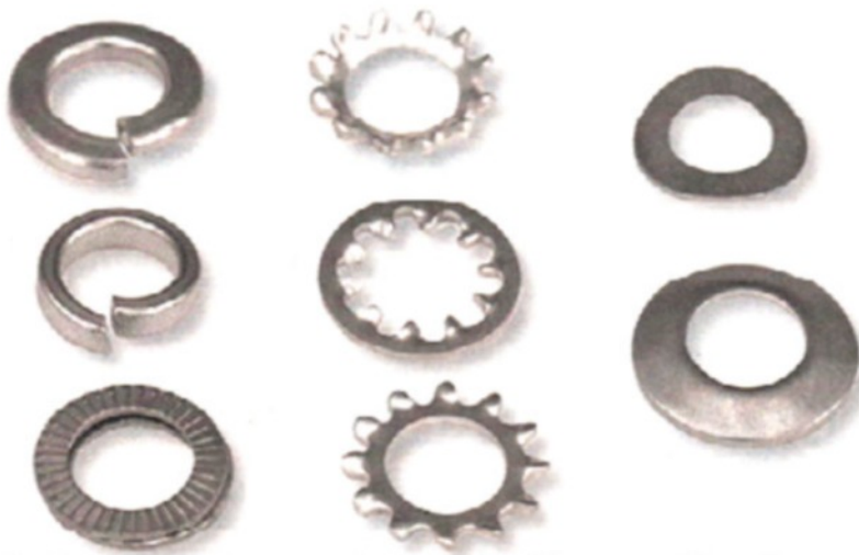
Lock washers come in a variety of forms – split washers in standard and high collar diameters (left middle and upper) toothed washers (middle) can have internal or external teeth and some are available for countersunk holes, and wave washers and Belleville are often found in light duty applications (right). The unique wedge lock washers are relatively new and are extremely effective (lower left).
